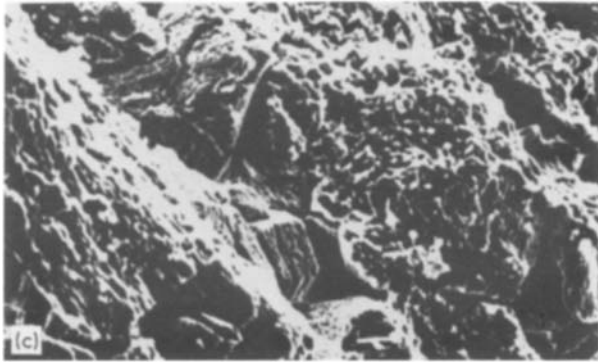
Figure 6 Scanning electron photomicrograph of alumina bodies annealed at 1500°C for (a) 25 h, (b) 50 h, (c) 100 h. Magnification: (a) and (b) \times 1700 , (c) \times 850 .
